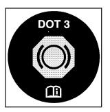
Your brake master cylinder reservoir is filled with DOT-3 brake fluid. See Engine Compartment Overview on page 5-14 for the location of the reservoir.
